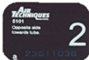
FIGURA 6: SENSOR PSP ( photostimulable phosphor plates ). TOMADO DE INTRAORAL IMAGING: BASIC PRINCIPLES, TECHNIQUES AND ERROR CORRECTION 2
