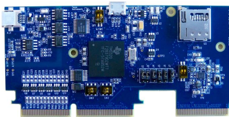
Figura 3.3: Imagen referencial de F28379D controlCARD for C2000 Real time control development kits.
