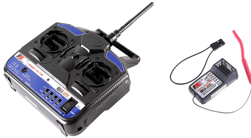
Fig. 1.2.4.6: Emisor-receptor de radio control.
